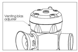
50/50 is reached. As you turn the adjuster further clockwise, the recirc port is fully open and the trumpet port will begin to close. When the adjuster reaches the maximum clockwise position, the trumpet is completely closed, and the valve will operate like a factory recirculating bypass valve.
